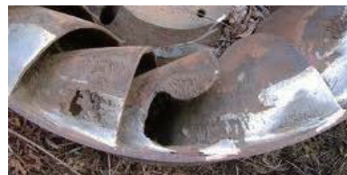
Marine propeller eroded by cavitation
