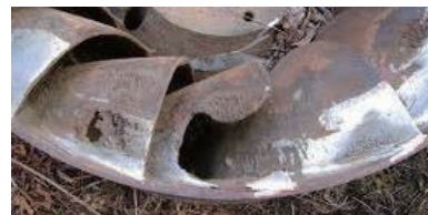
Marine propeller eroded by cavitation
