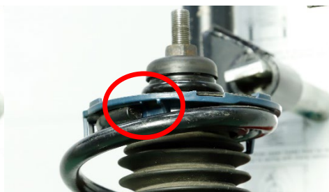
This is typical wrong phase of Coil spring!!! Makes some noise.
