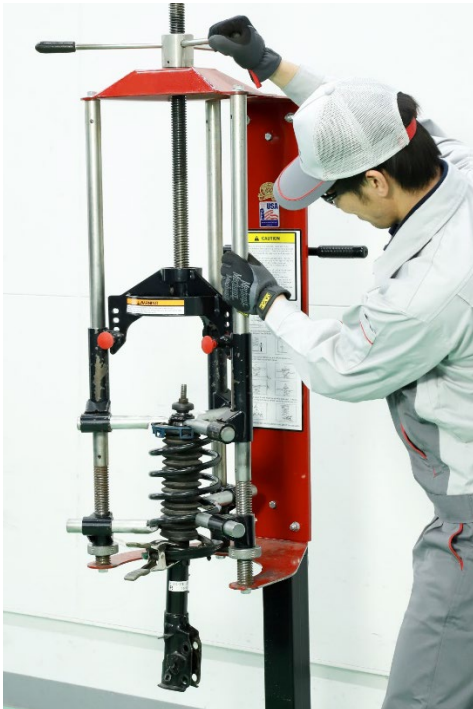
Perfect! There is no space between end of coil spring and seat rubber
