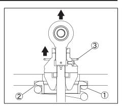
4. Remove the spring seat stopper ② and the spring ①, and replace the spring.
