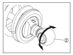
The line of the screw part ③ of the lower metal ② is the reference line. When set in the center of line ③, the whole length of the BFRC<sup>®</sup> lite Kit is the reference dimension.
