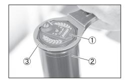
Pour operation fork oil into inside of the fork tube.
