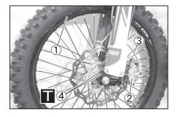
Tightening torque: 20 N·m
