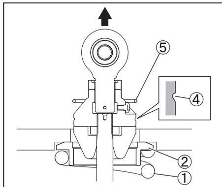
4. Check the spring seat stopper ② is hooked on the stopper ring ⑤, and remove the BFRC® lite Kit from the spring compressor.
