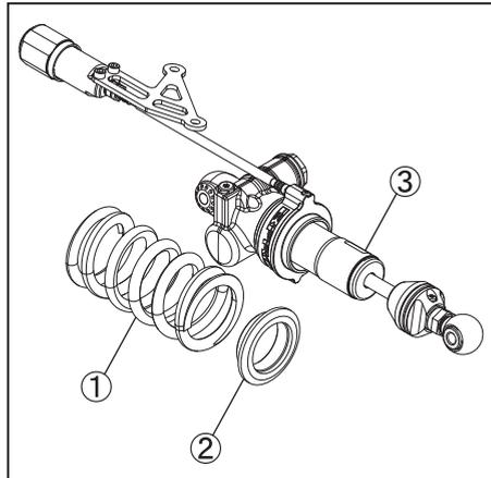
2. Attach to a spring compressor, and push down the spring seat stopper ② until the groove ④ is visible.
