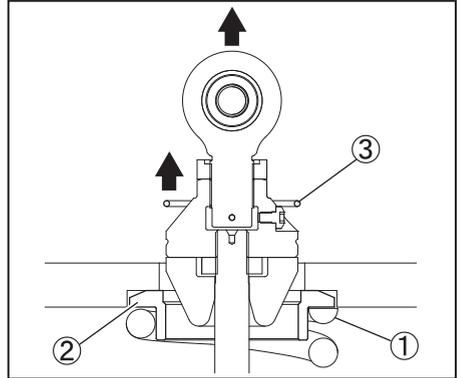
4. Remove the spring seat stopper ② and the spring ①, and replace the spring.
