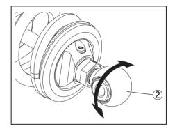
The line of the screw part ③ of the lower metal ② is the reference line. When set in the center of line ③, the whole length of the BFRC® lite Kit is the reference dimension.
