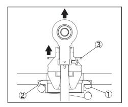
4. Remove the spring seat stopper ② and the spring ①, and replace the spring.
