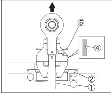
Check the spring seat stopper ② is hooked on the stopper ring ⑤, and remove the BFRC® lite Kit from the spring compressor.
